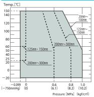
Use after confirmation that maximum operation pressure and maximum ervice temperature is within the operation range.
